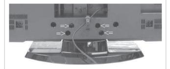
Remove the 4 stand fixing screws indicated and lift the TV set up and away from the 'Stand Assy'.
