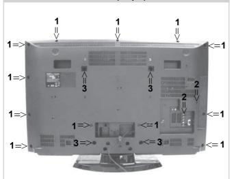
Remove the rear cover fixing screws indicated and refer to Sec 2-2-2.
