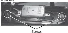
To remove the 'Loudspeaker' first disconnect the speaker cables and then remove the screws circled (32/37" = 4 pcs, 40" = 2 pcs).
