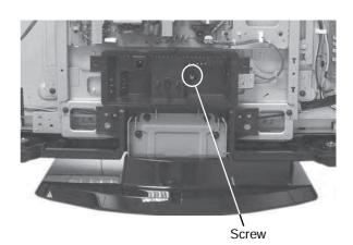
To remove the 'Under Cover' first remove the Rear Cover (See Sec 2-2-1 & 2-2-2) and then remove the Stand Assy (See Sec 2-2-3). Then remove the 1 screw circled and gently pull the 'Under Cover' away from the back of the TV set.
