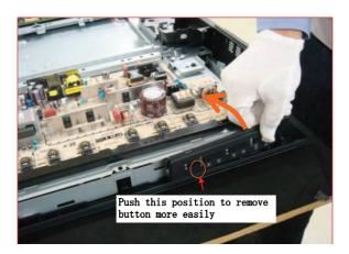
To remove the 'Switch Unit' lift the bottom of the bracket towards the TV set. Push the top of the bracket in the shaded area in the photograph. The bracket will then release from its boss and can be removed from the TV set.
