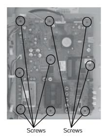
To remove the 'B' board disconnect all the connectors and then remove the 9 screws circled and ease the board gently away from the back of the TV set.
