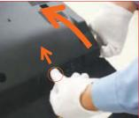
To remove the 'Rear Cover' lift the 'Rear Cover' up slightly from the bottom and then gently push the 'Switch Unit' in by the side controls whilst lifting the 'Rear Cover' up fully from the bottom.
