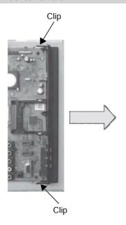
Release the 2 clips indicated and gently pull the bracket away from the 'B' board in the direction of the arrow.
